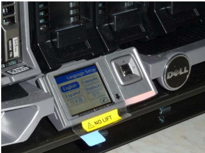
Use the silver arrow pad to the right of the LCD screen to move to a selection. Press the center of the silver pad when you are ready to confirm your choice.
